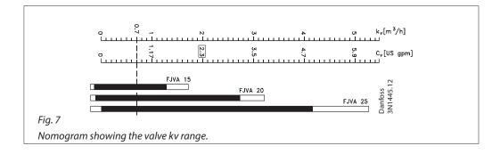
$K_{_{\rm v}}$  values are always given for water flow in [m³/h] with a pressure drop  $\Delta$ p of 1 bar. The valve should be selected so that the necessary  $k_{_{\rm v}}$  value lies in the middle of the regulation range.
