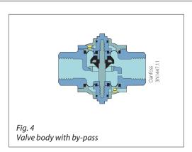
FJVA valves are for applications where, because of installation problems, etc., it is desirable to avoid using a capillary tube. This applies mainly where regulation accuracy requirements are more moderate and where an integral bypass can be accepted.
